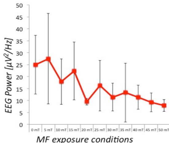
Fig. 4. Average EEG Power in the alpha frequency band (8-12 Hz – O2 electrode) in 1 preliminary subject as a function of MF flux density conditions – global head exposure. It shows a noticeable trend towards a decrease of EEG alpha power as the MF flux density increases.
