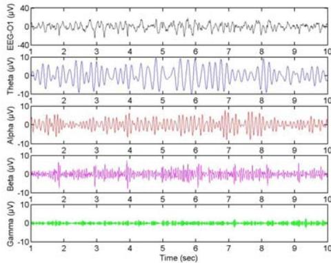
**Figure 2:** From the top to the bottom: 10 sec of O1 EEG trace and corresponding theta, alpha, beta and gamma components respectively extracted using FFT and iFFT. Averaged amplitude for this sample are: Theta = 3.909  $\mu$ V, alpha = 2.485  $\mu$ V, beta = 1.757  $\mu$ V; gamma = 0.641  $\mu$ V.
