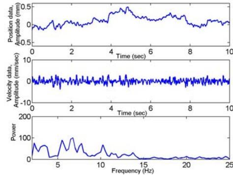
**Figure 3:** Position data (top), velocity data (middle) and corresponding power spectrum (bottom) for 10 sec of recording during MF exposure with eyes open (block 3). The computed values on this sample are: Amplitude = 0.032 mm; drift = 0.106 mm, median frequency = 7.04 Hz; and frequency concentration = 6.31 Hz.
