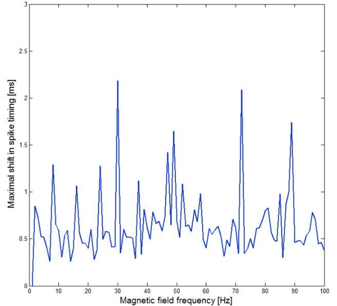
**Figure 2:** Role of the ELF MF frequency on the perturbation of spike timing as measured by the maximal SST.
