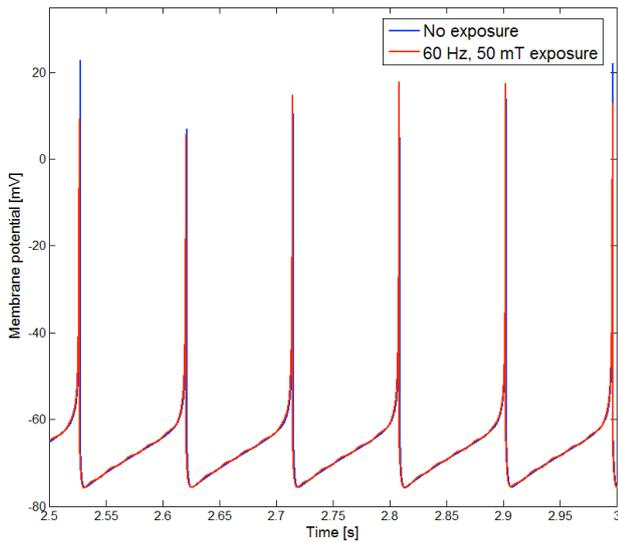
**Figure 1:** Membrane potential of a regular spiking cortical neuron during exposure to an ELF MF of frequency 60 Hz and amplitude 50 mT.
