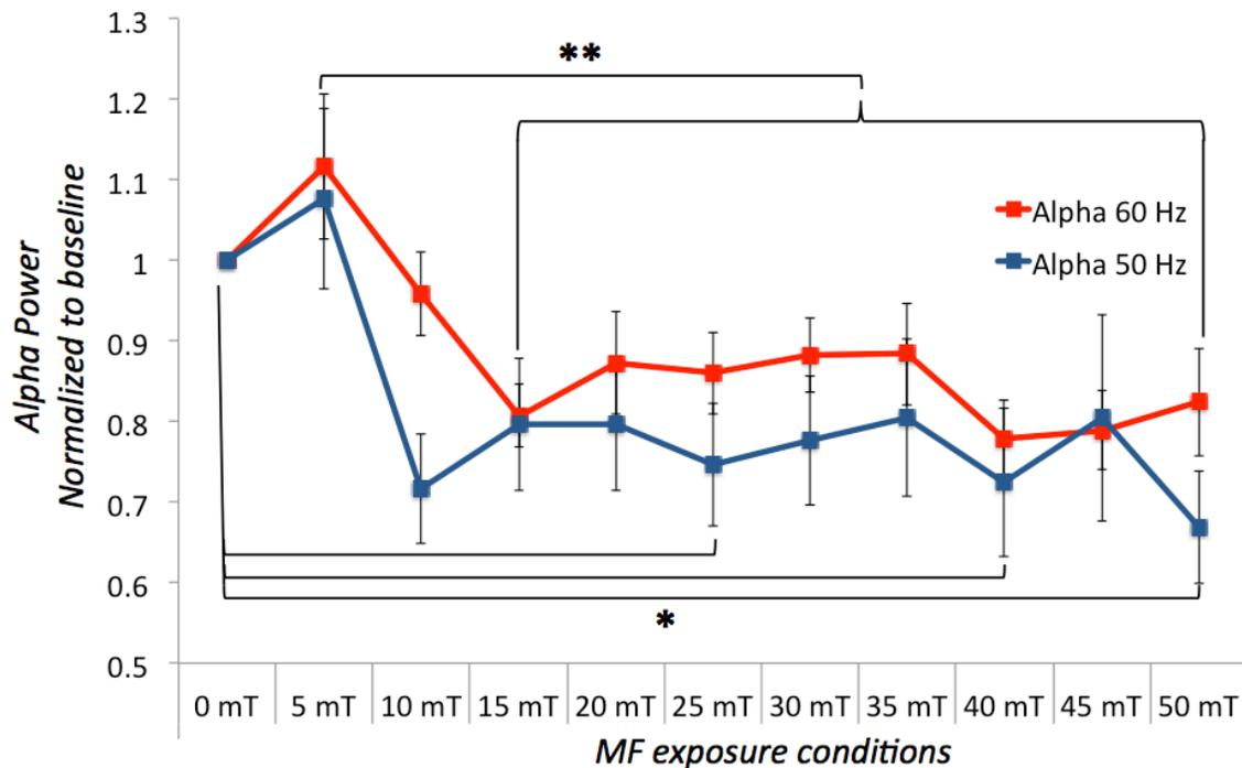
**Figure 2:** Evolution of the EEG alpha power in the global exposure condition at 50 (n=25) and 60 Hz (n=26) for MF flux densities between 0 and 50 mT. Above 15 mT, EEG alpha power is becoming significantly decreased, i.e. above the magnetosphene detection threshold.
