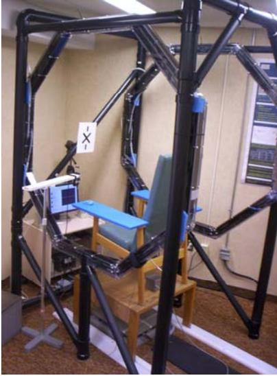
**Figure 2:** The elevated armchair installed between the two coils of the exposure system. The head of the subject was located in the homogeneous MF region.
